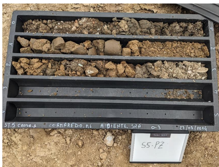
Figura 10 – Piezometro S5-PZ (0.0 – 3.0 m)
