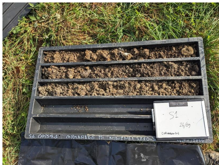
Figura 2 – Sondaggio S1 (0.0 – 3.0 m)
