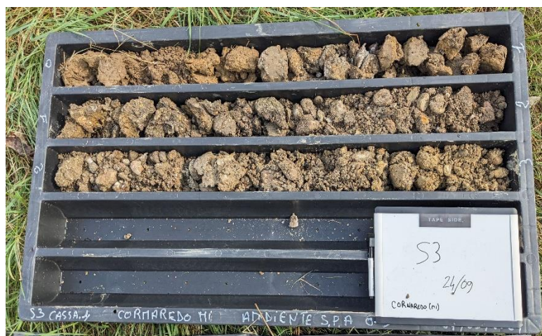
Figura 4 – Sondaggio S3 (0.0 – 3.0 m)
