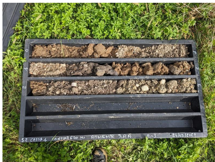
Figura 8 – Piezometro S2-PZ (0.0 – 3.0 m)
